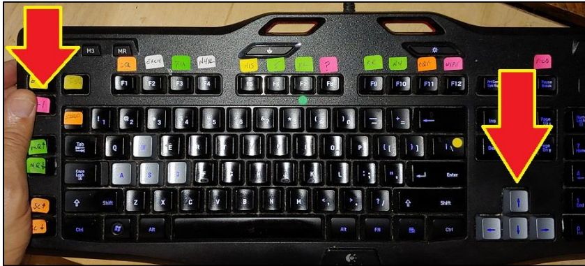
Fig. 1 Gaming Keyboard showing access to programmed macro buttons on left and up/down arrows for changing frequency on right
