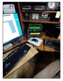
Good station ergonomics includes making controls you use frequently easy to access. I have my TS590's right next to the keyboard and mouse, the paddles and SO2R box at hand, and the antenna switches and rotor right above them to allow ease of use. They are all within easy eye and head movement of the computer screens which minimizes the muscle strain that inevitably comes with a 30+ hour contest effort.
