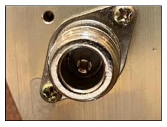
Here are a couple of before and after photos. Unfortunately, I had already gently moved the fingers back into position in the before photo but you can still see the fingers were slightly splayed apart before the addition of the tubing.
