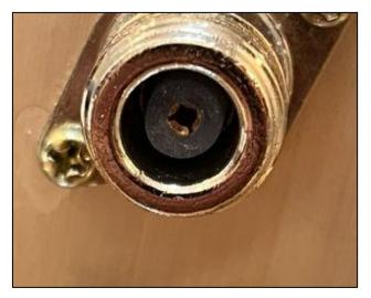
Here is a photo after the tubing has been installed over the center pin receptor.
