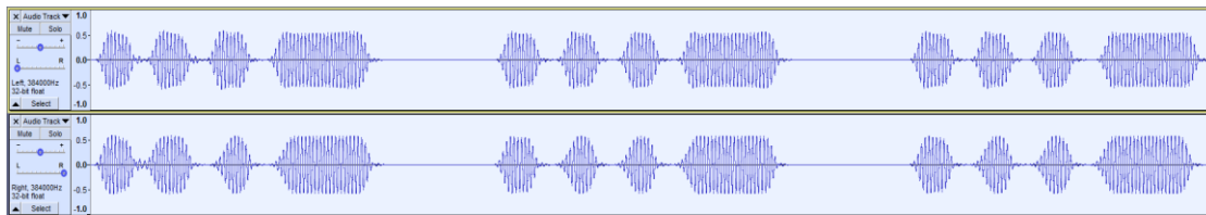
Figure 12: 60 WPM Rx Audio of the IC-7300 Tx signal: 2ms Rise time (top) and 8ms Rise Time (bottom)
