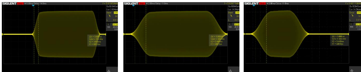
Figure 3: Keying of the K3 at 20WPM (l/h), 40WPM (center) and 60WPM (r/h)
