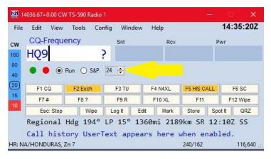
This area shows my selected CW speed (24 WPM), that I am in Run instead of S&P mode (you may have different macros for each), and the receive/transmit focus/status. The latter is used for SO2R setups. The red dot turns orange if you are transmitting using that particular entry window
