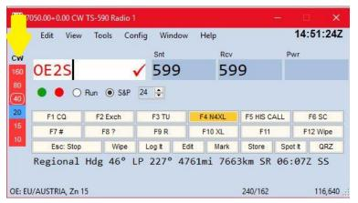
The band area shows the rig is on 40 meters (the white circle around 40), that OE2S is a multiplier on that band (because the 40 is red), that he is also a mult on 160, 80, 15, and 10 (They are all red), that even though he is not a multiplier on 20 (it is blue) I can work him for points there (if it was gray it would mean I have already worked him on 20). You can use this information to try and pass him to another band
