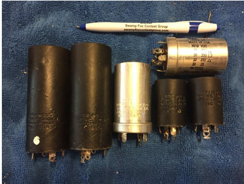
Above are the old electrolytic capacitors from the Drake TR-4 and its accompanying power supply.
