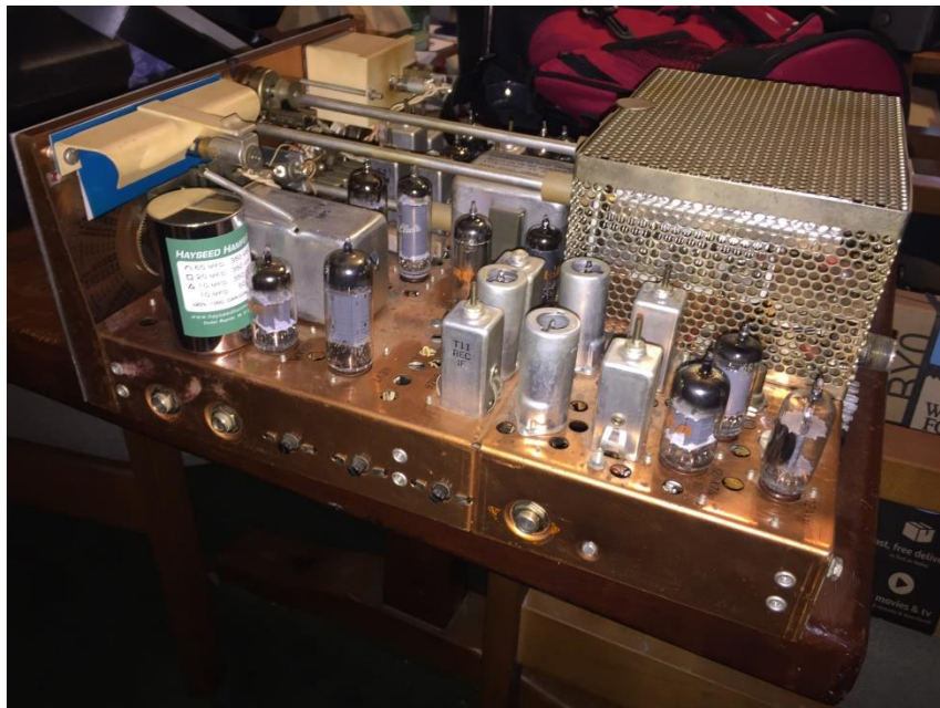
A look under the hood of the rig, with the new capacitor canister installed.
