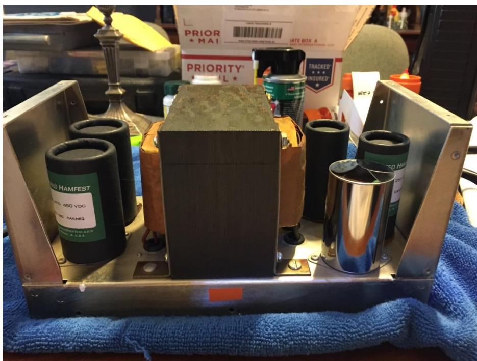
This is the power supply with the new electrolytic's installed.
